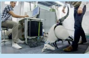
We jumped at this opportunity to get our kangaroo out of the starting block. Our point of departure was a single leg that we fitted out with a pneumatic cylinder to give it the necessary bounce. We attached the leg to a treadmill mechanism with angular sensors and made it hop around in circles. At first we controlled the air valve by hand to get a feel for its operation: at what point in time and in what rhythm are the jumps performed the most successfully?
