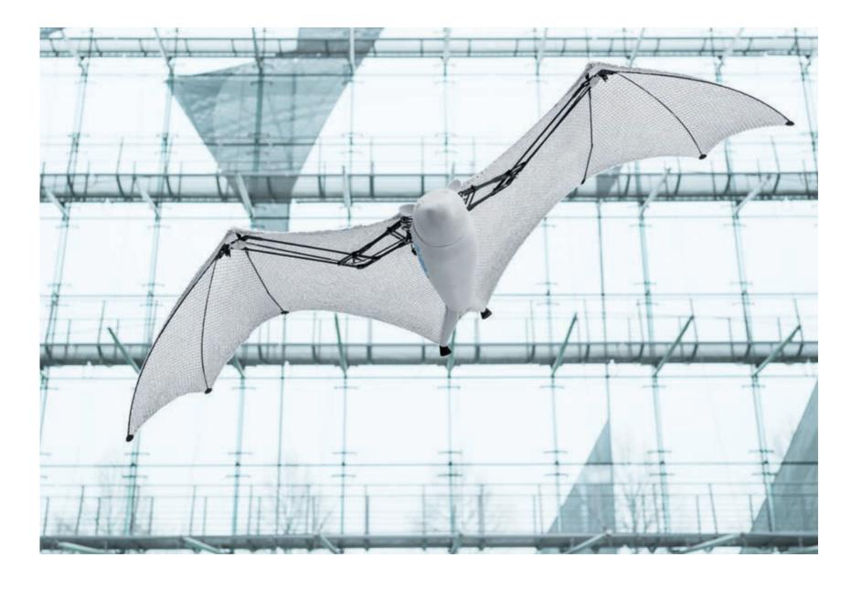
Innovative flying membrane of knitted elastane textile covered with foils: the honeycomb structure enables the BionicFlyingFox to fly even in case of minor damage to the textile
